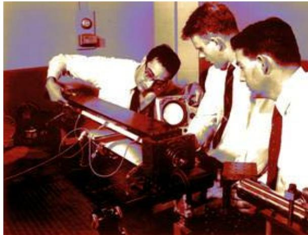
*1960:* **Ali Javan, William Bennett, and Donald Herriott adjust the helium neon laser, the first laser to generate a continuous beam of light at 1.15 microns and the first of many electrical discharge pumped gas lasers.**
